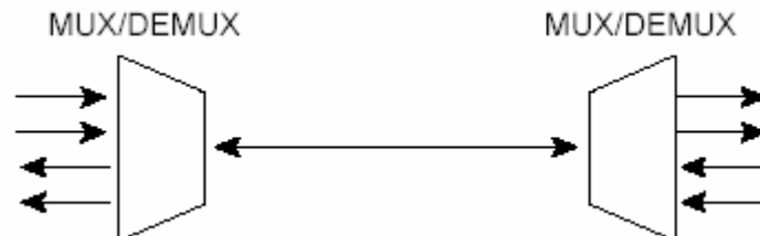
Figure 17-10 Multiplexing and Demultiplexing in a Bidirectional System
